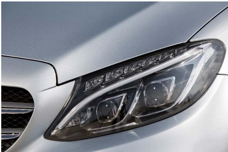
Headlamps add distinction to the front of a car, illuminate the road surface, and make the vehicle visible to other road users. In the LED Intelligent Light System of Automotive Lighting, which Mercedes-Benz is installing in its current Mercedes-Benz C-Class, three different PLEXIGLAS® and PLEXIMID® molding compounds are used. Source: © Daimler AG
