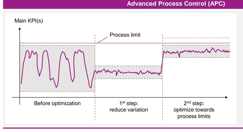
**APC optimizes** complex production processes under consideration of many process parameters and ensures production at the **ideal operating point**
